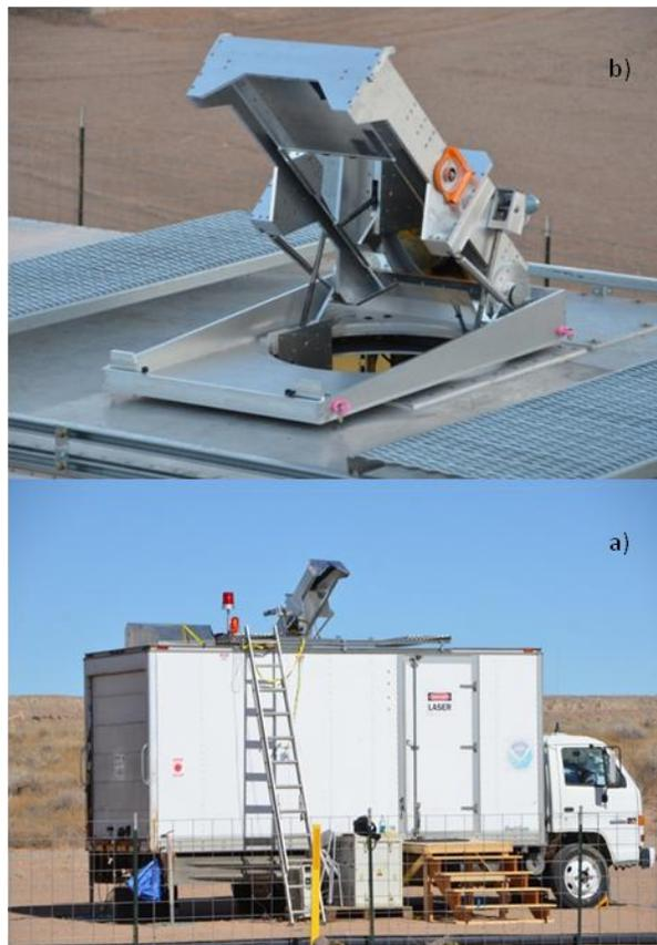
Figure 2. a) TOPAZ deployed at the UBWOS experiment. b) Detail of scanner.
