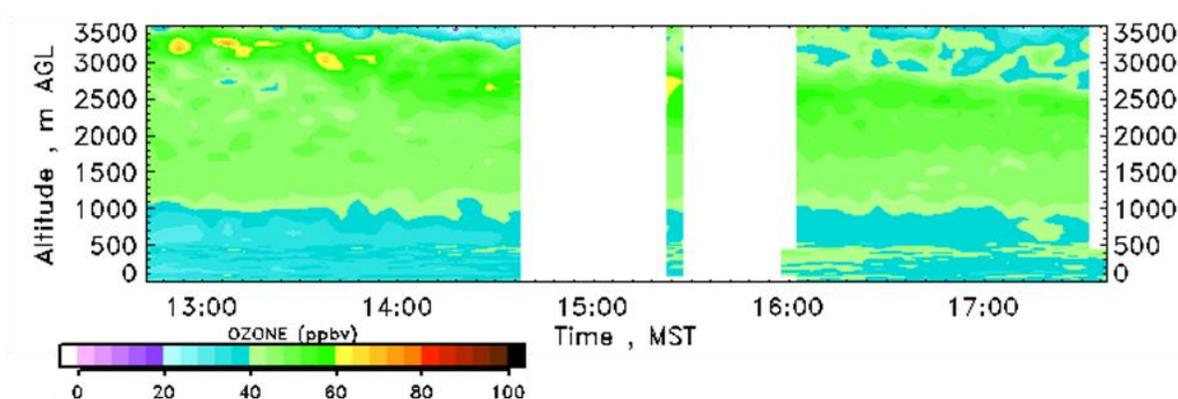
Figure 4. Time-height cross section of ozone concentration from the UBWOS experiment. The individual profiles are composites from three angles as shown in Figure 3, and the concentration is indicated by the colors as shown on the color bar.
