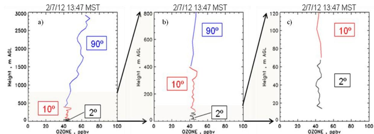
Figure 3. Composite profile of ozone concentration from the UBWOS field experiment. a) Entire profile (15-3000 m above ground level) with each segment labeled according to the lidar pointing angle that the data is derived from. b) The lowest 800 m expanded to show the higher resolution in the lower altitudes. c) The lowest 120 m expanded.
