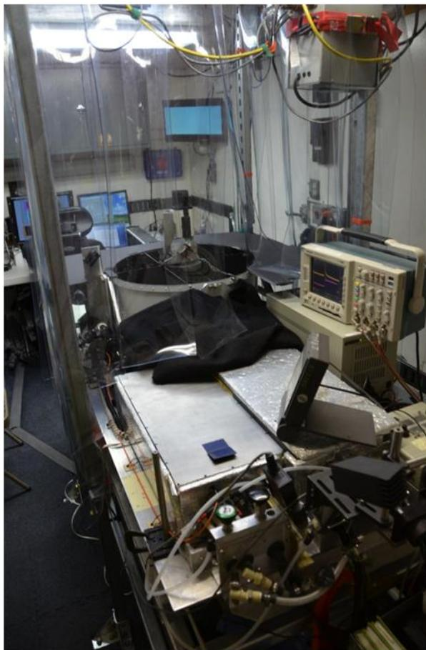
Figure 1. The TOPAZ lidar system reconfigured with up-looking telescope and installed in its truck platform.
